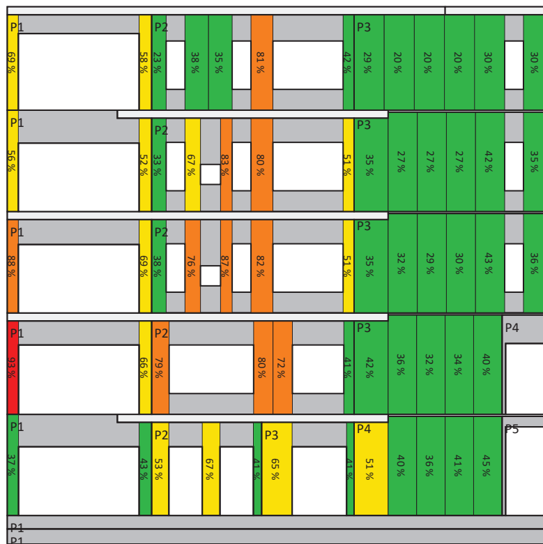
Figure 135: Critical wall slices. Utilization.
