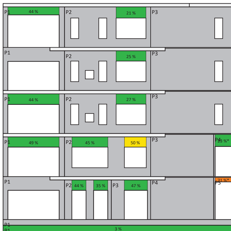
Figure 148: Critical utilization of beams across all load combinations.
