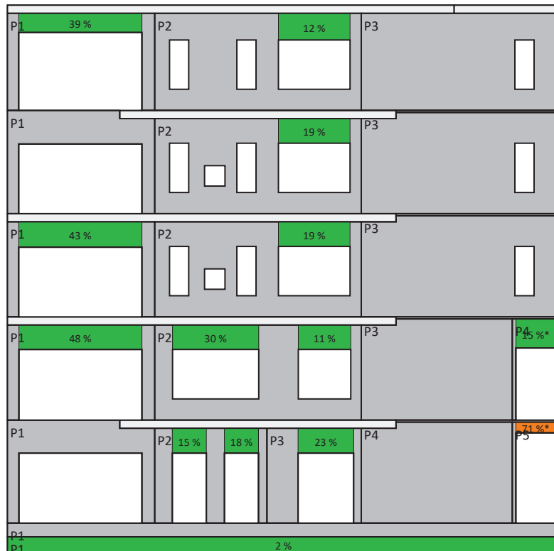
Figure 150: Utilization of beams in load combination: 6.10b 1.5 qk + 0.3 wk+ + gsup.
