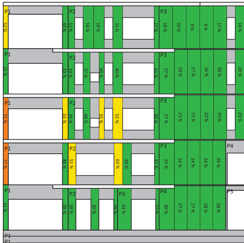
Figure 137: Utilization of wall slices.
