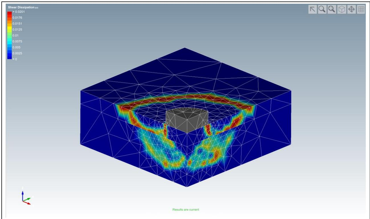
Figure 2: Shear dissipation (shear stress x shear strain) at failure for Mixed element
