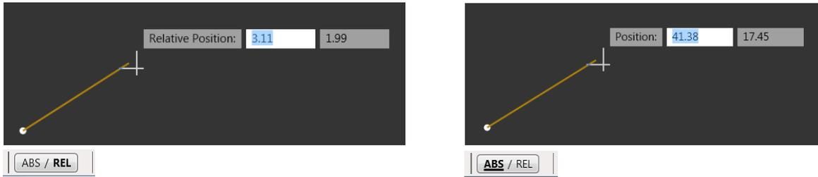
Figure 3: Relative (left) and absolute (right) coordinate input modes.
