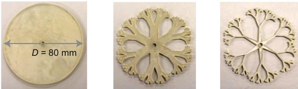
Figure 56.1: Standard circular and fractal anchor plates (after Dyson and Rognon 2014).
